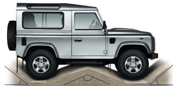
Departure angle Ramp angle Approach angle
